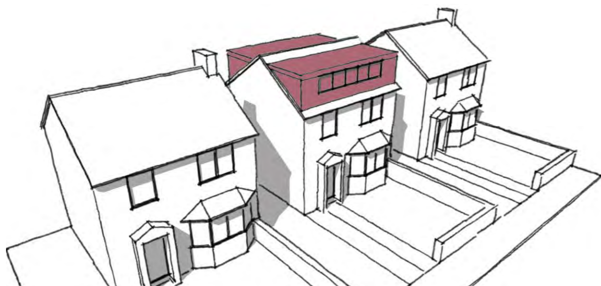
Figure 304: Example of an unacceptable dormer
